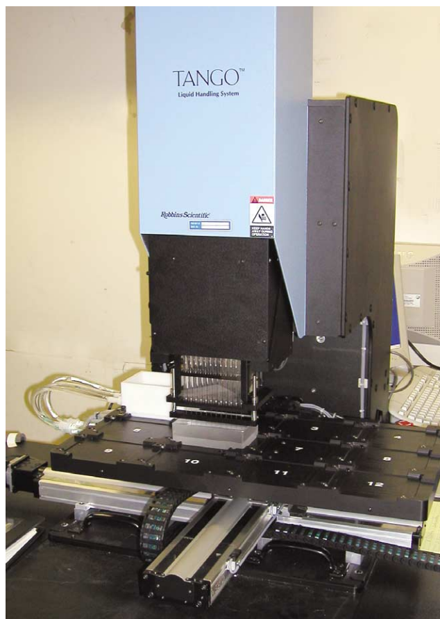
Fig. 3. The Apogent Discoveries, Robbins Scientific Tango liquid handling system is very well suited for delivery of solutions to set up 1536-well plates containing microbatch-under-oil crystallization experiments. The LHS is made up of an exchangeable delivery head. The head can hold an array of 1, 12, 96, or 384 syringes. The syringes work in unison to aspirate or dispense solutions from a source to a destination plate. The plates are held in position on an xy translation stage that moves beneath the syringe bank head. The entire system is controlled through a GUI that permits the user to define all aspects of the delivery protocol.
