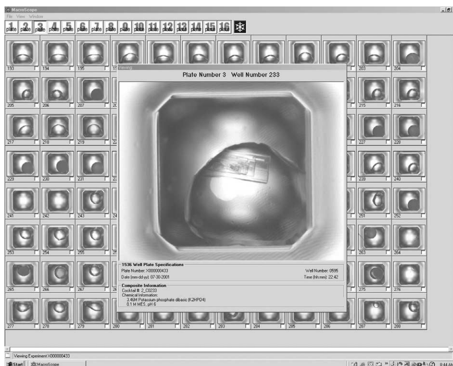
Fig. 5. MacroScope is software designed to view the results of the 1536 microbatch-under-oil crystallization experiments. The software displays 16 groups of 96 thumbnail images. When an image is selected it will expand to full size and provide information on the time the image was recorded and the chemical information about the cocktail solution.
